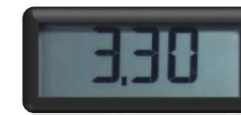
Fig. 5d: Shunt Regulator T C = 65.2°C at V IN = 60V DC Above: V OUT still stable at 3.3V
