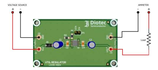
Use the following steps to connect the evaluation boards to a voltage source and an ampere meter:
