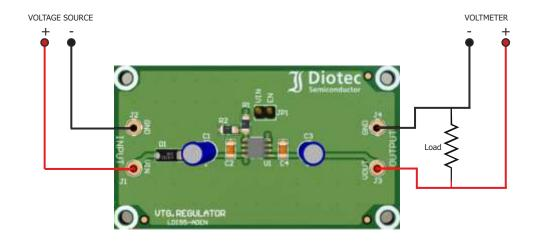
Use the following steps to connect the evaluation board to a voltage source and voltmeter:
