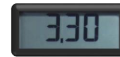
Fig. 5d: Shunt Regulator T_c = 65.2^\circ\text{C} at V_{IN} = 60\text{V}_{DC} Above: V_{OUT} still stable at 3.3V
