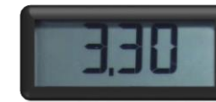
Fig. 5c: Shunt Regulator T_c = 55.4^\circ\text{C} at V_{IN} = 10\text{V}_{DC} Above: V_{OUT} stable at 3.3V
