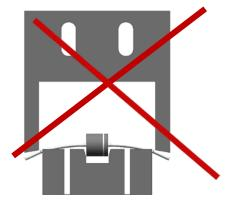
Mechanical stress is applied through lead wires to semiconductor crystal
