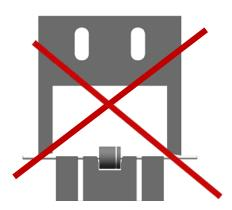
Cutting/bending without strain relief!
