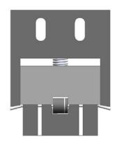
Step 2: Cutting/bending with strain relief √
